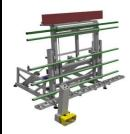
• 2 cylinders for tilting table, another 2 for conveyor's lifting up and another 3 for regulation of working top's level,
